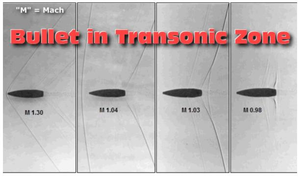
These four photos show the substantial changes in the shock wave and turbulence patterns for the same 7.5mm bullet at different velocities. The "M" stands for Mach and the numerical value represents the velocity of the bullet relative to the speed of sound at the time of the shot. Photos by Beat Kneubuehl.
